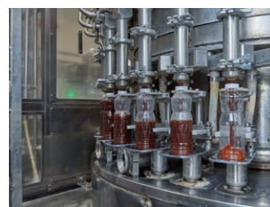
Filling process: Bottle and cap the sauces which sterilized with heat.
