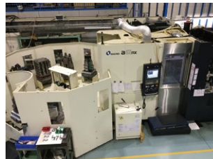
7-hedral pallet type horizontal machining center This multi-hedral pallet type machine allows for continuous processing for many hours. Number of cutters: 130.
