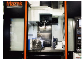
Vertical machining center (5-axis type) A vertical machining center equipped with a tilt indexer and an automatic tailstock.
