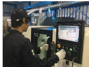
CNC composite machine A cutting-edge composite machine which has a numerically controlled lathe and a milling device.
