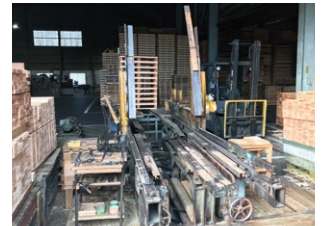
Forth machine A semi-automatic nailing machine for producing four- and two-sided pallets.
