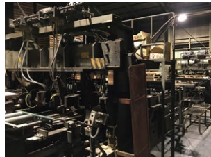
First machine A Fully automatic nailing machine which can accept wood from 1000 to 1500 mm
