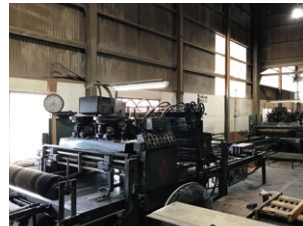
Third machine Made by Viking (USA): an automatic two-sided nailing machine.
