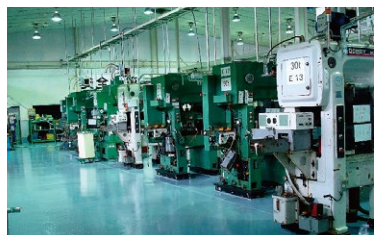
Progressive pressing facilities: from 5 to 300 tons (40 units in total).
