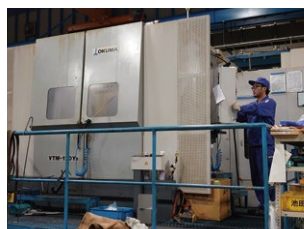
Composite turning center A function-aggregation type vertical composite processing machine which can process polyhedral parts.
